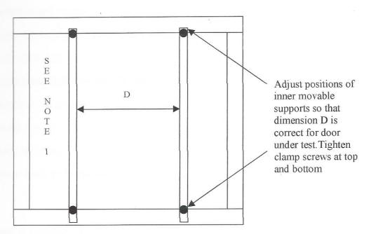
NOTE 1 If door under test is narrower than the outer frame fill gaps at either side to restrain air bag.
