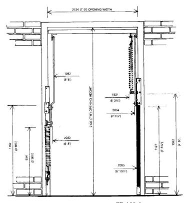
standard retractable gear CD150,200,250 CD 100 door gear (on doors up to 8'0 x 7'0)
